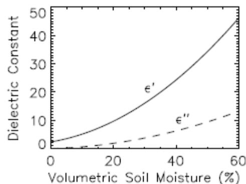
Figure 1.5: Dielectric constant  $\epsilon$  for a loamy soil versus the volumetric soil moisture content in percentage
