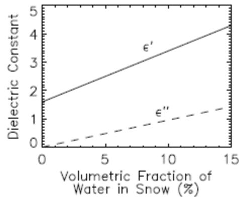
Figure 1.7: Dielectric constant  $\epsilon$  of snow versus the volume fraction of water in percentage
