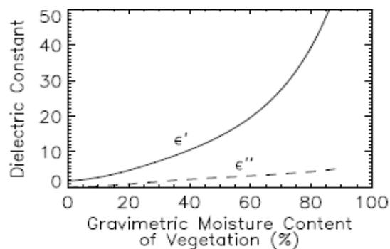
Figure 1.6: Dielectric constant ( $\epsilon$ ) of vegetation versus the gravimetric soil moisture content in percentage
