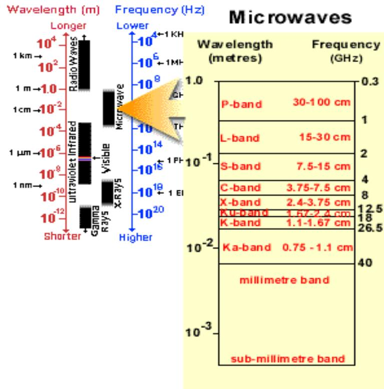
Figure 1.1: Position of Microwaves in the Electromagnetic Spectrum [62]
