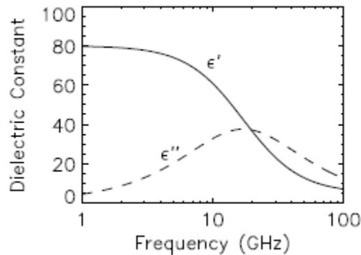
Figure 1.4: Dielectric constant  $\epsilon$  of pure water versus frequency at 20<sup>0</sup> C
