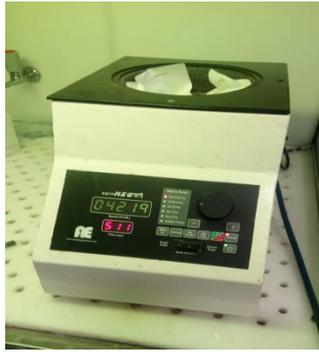
Fig. 4.9. Photograph of the spin coating machine used (spin NXG-M1) [courtesy-microfabrication lab facility, Tezpur University].
